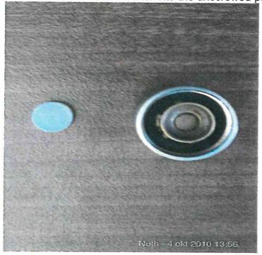
Step 5. Put the white ( in some case it can be a black part ) sealing in the open part of the waterbreaker. From now on this part is available as a spare part.
