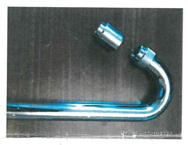
Step 2. Remove the different parts from the part that you have unscrewed. The part that is white on this picture is in real black and it is the main part that takes care of the sealing of the tap. ( It is mostly the cause of the dripping ).
